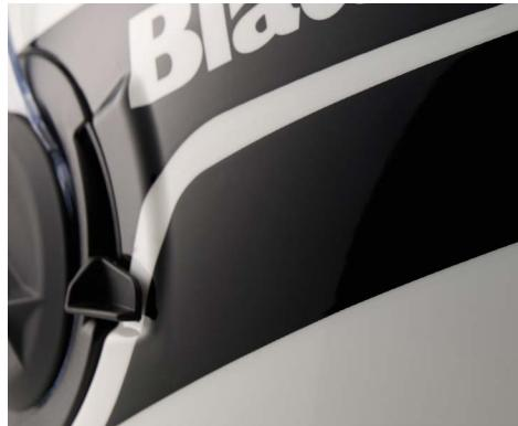
The sun visor lowers moving the sun shield slider from the top down.
